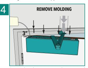
Once you have the measurements down, position the operator and screw into position. Remove molding for flush mounting against the wall.
