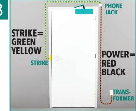
Strike Connection: Connect Green and Yellow wires from phone jack to strike. Power Connection: Red & Black cables need to run from phone jack to transformer. Transformer is then plugged in to 120VAC wall outlet.
