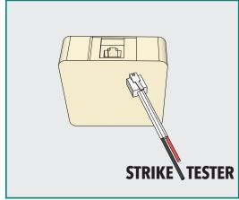
Plug in Strike Tester to RJ-11 phone jack to test electric strike, you should hear a buzzing sound coming from the strike (Do NOT connect any wires to this tester).
