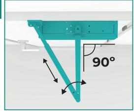
With the door closed, adjust the arm to 90 degrees.
