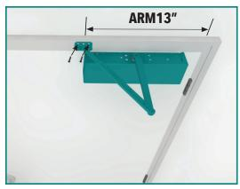
Line up the arm with marking you did on the door jamb so that the middle of the shoe is position where the mark is, then screw into place. Do NOT mount arm shoe too high above operator because it will cause binding of joints leading to screws falling off.
