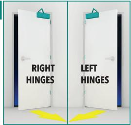
Operator will need to be on the top corner closest to the hinges.
