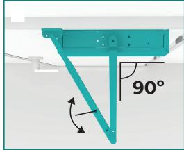
After setting up the correct adjustment tighten the arm with the supplied 4mm allen wrench.
