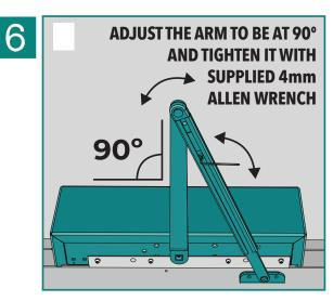
Note: Position Model 133 at 3" and Model 233 at 4" away from hinges and mount arm at 13" from hinges. Mount arm shoe  $1\,^3/_8$ " down from top of the door. After mounting unit, see page 9 and review instructions on inside cover.
